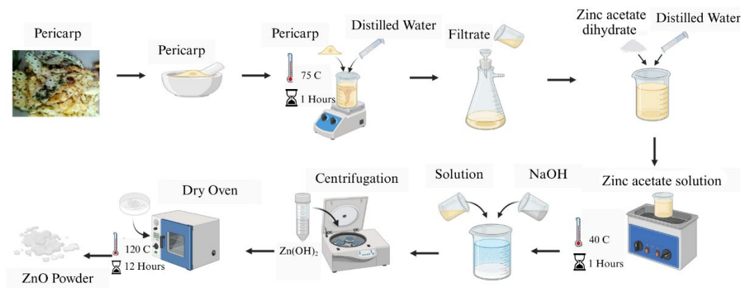
Figure 1. Synthesis procedure of ZnO nanoparticles
